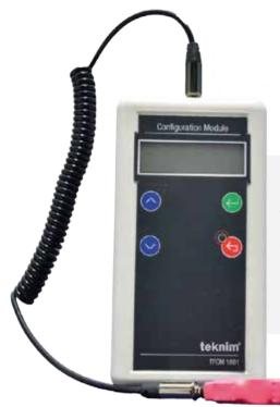
TFCM-1801 device programming module is developed to define address for addressable devices such as detectors, mcp, input-output modules or to read defined address and firmware version of the devices. It is supplied from 9V (6LR61) battery.
