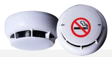
TFD-3940 and TFD-3945 are battery operated detectors which can be used stand-alone in to detect fire alarm. While TFD-3940 supports multi sensing technology with optical and heat, TFD-3945 supports cigarette smoke and heat sensing technology.
