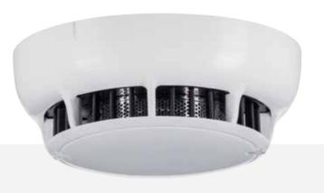
TFD-3240 Conventional fixed heat detector uses two NTC for precise measurement of the environment to detect fire. Detector classified as A2S and will report an alarm at 55°C.
