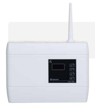
Teknim TWM-3885 Conventional Coordinator is an interface device that enables wireless devices to be operated with conventional fire alarm panels. The Wireless Conventional Coordinator module, which can work in full compatibility with all brand and model conventional fire panels by using the desired end of line resistor, processes the signals it receives from all wireless devices and enables the warning and notification functions in the control panel.
