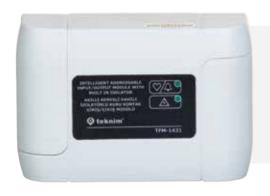
TFM-1431 used with TFP-12xx series addressable fire alarm panels and supports single input and output. The device is also supporting built-in isolator to protect the loop line against short circuit.
